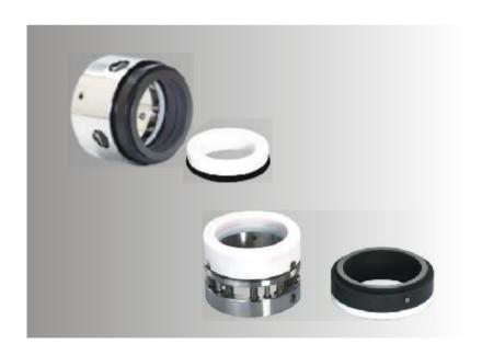
The PM-Series Seals are designed to handle clear liquids and generally accepted in the seal market by the OEM's. The transmission of the torque from the retainer to the seal ring is done by the drive lugs. And to make the installation easier. All the components are held together with a snap ring. These seals are also offered in balanced and unbalanced versions which depend upon the pressure parameters.
