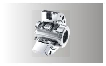
A cartridge type mechanical seal is a pre-assembled package of seal components making installation much easier with fewer points for potential installation errors to occur. A Cartridge Seal assembly is "pre-set" so that no installed length calculations must be performed for determining where to set the seal. Only the external seal in a double cartridge have "set tabs" that are removed once the seal is installed and the pump assembled.
