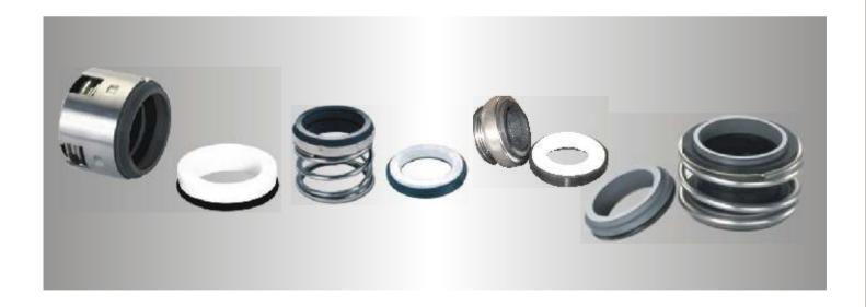
The PEB Series seals are low cost rubber bellow seals which can be used for non critical applications like water. The heart of the seal is the flexible rubber bellow made from Viton, EPDM, NBR etc.. Based on the applications the Seal faces can be offered in Carbon, Tungsten carbide, Silicon carbide, ceramic etc.. The salient features of the above seal is no need for skilled manpower for installation.
